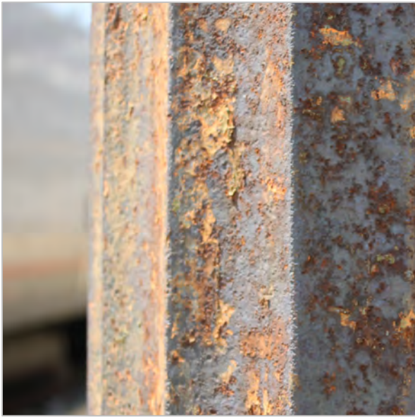
SURFACE CORROSION
