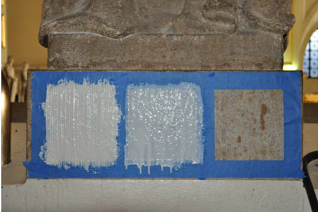
Figure 12. Applied mockups. L-R MasonRE, Dri-Klean, & dry soot sponge.
