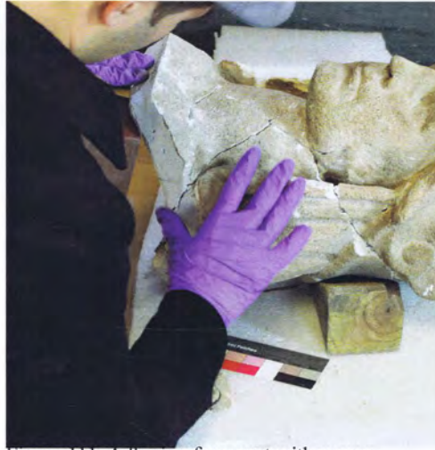
Figure 111. Adhering fragment with epoxy.
