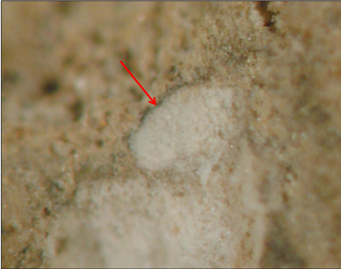
Photo 6: Cross-section view at the exposed surface of sample PA01, 63x. The tan material is the coating; the white is the binder. The thin black line between (red arrow) appears to be a dirt layer.
